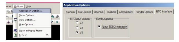
Ensure that "Allow EDMX reception" is checked, and that the ETCNet2 Version is set to V4. Note: You must restart WYSIWYG after making this change. You also must be an Administrator on the computer.
